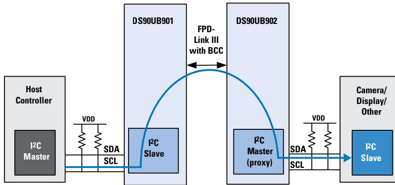
**Figure 5. Accessing a Remote I<sup>2</sup>C Slave Using the FPD-Link III Bidirectional Control Channel**
