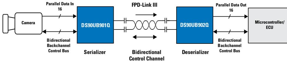
**Figure 1. A Typical LVDS-Based SerDes Chipset Connects a Camera to an ECU**
