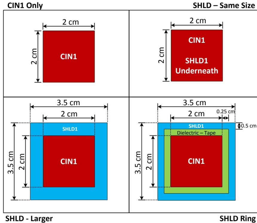
Figure 9. Sensor Layouts - Top View
