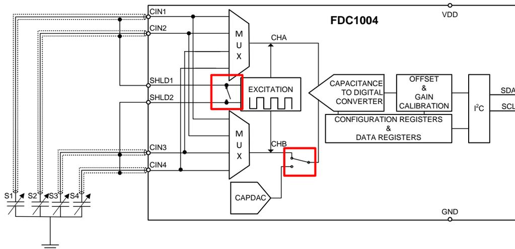
**Figure 8. Shielding in Differential Configuration, CAPDAC Disabled**
