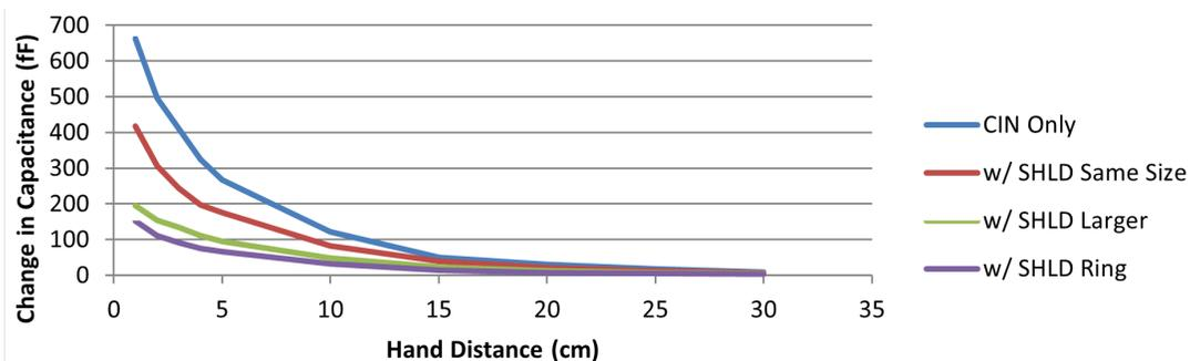
**Figure 15. Experimental Results of Proximity From the Side**
