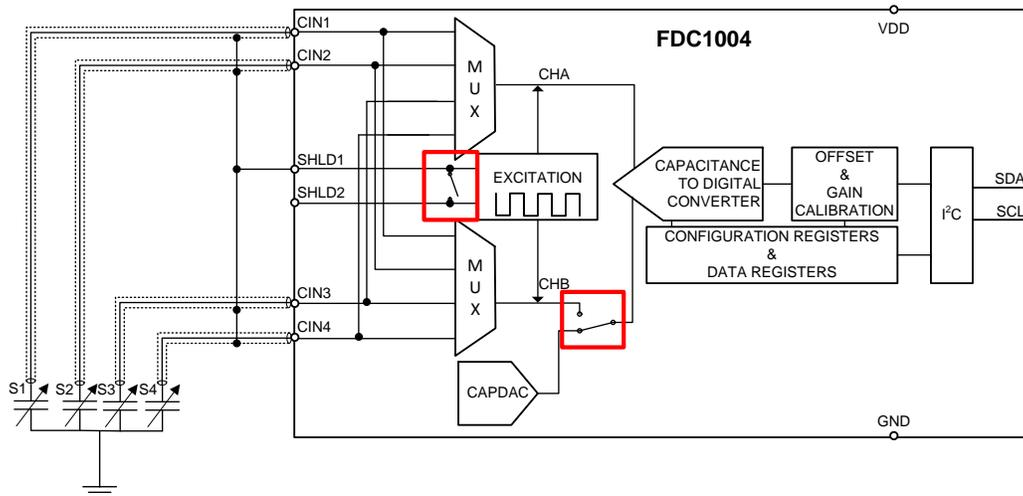
**Figure 7. Shielding in Single-Ended Configuration With CAPDAC Enabled**
