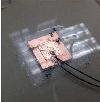
Figure 11. Actual Sensor - Larger SHLD1 Underneath CIN1
