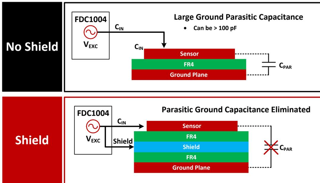
Figure 4. Ground Plane Effects With and Without Shielding
