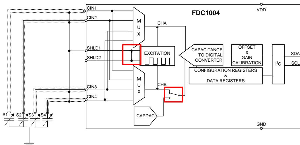
Figure 6. Shielding in Single-Ended Configuration With CAPDAC Disabled
