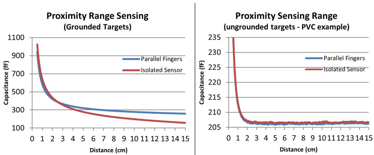
**Figure 3. Capacitance vs Distance Comparison for Grounded and Ungrounded Targets**
