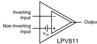
**Figure 1. Voltage Offset Modeling**
