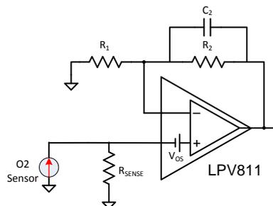
Figure 7. Oxygen Sensing Configuration
