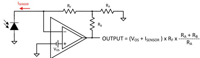
Figure 13. Transimpedance Amplifier with Feedback-T
