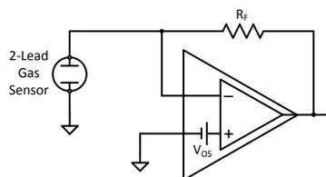
**Figure 12. Carbon Monoxide Sensing Application**
