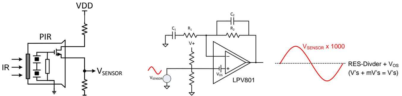
Figure 6. AC-Signal Amplification
