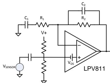
Figure 4. Non-Inverting Amplifier with AC-Gain ONLY
