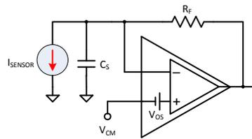
**Figure 10. Transimpedance Amplifier Configuration**
