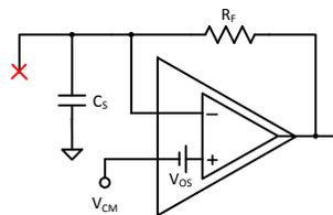
**Figure 11. Simplified Circuit After Applying Superposition**
