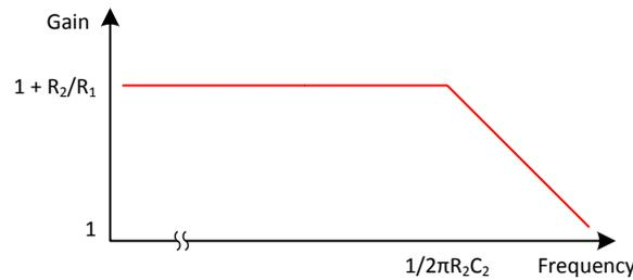
Figure 8. Bode Plot of DC-Coupled Signal
