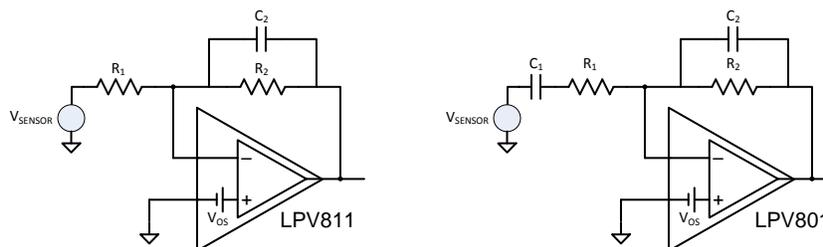
Figure 9. Inverting Amplifier Configurations
