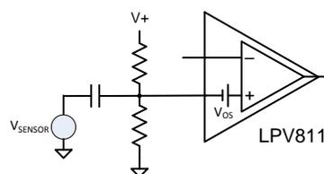
**Figure 3. AC-Coupling Input Signal**
