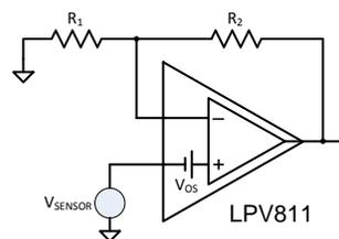
**Figure 2. Non-Inverting Amplifier Configuration**
