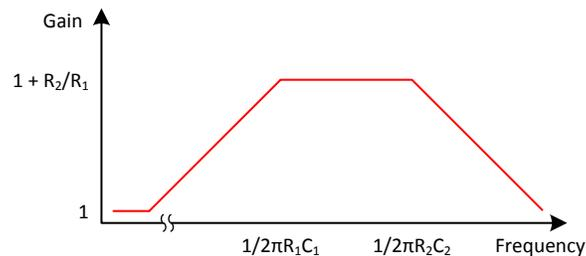
Figure 5. Bode Plot of Non-Inverting Amplifier
