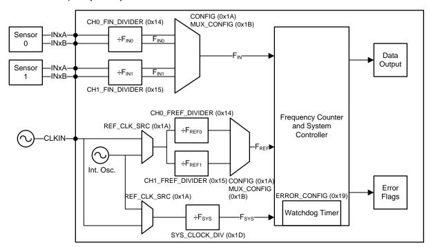
Figure 1. LDC161x Clocking Diagram
