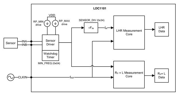
Figure 2. LDC1101 Clocking Diagram
