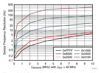
Figure 5. LDC161x Resolution with  $f_{REF} = 40 \text{ MHz}$
