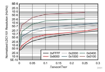
Figure 3. Normalized Frequency Resolution of the LDC161x vs f<sub>SENSOR</sub> and RCOUNT
