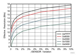
Figure 6. Effective Resolution vs RCOUNT and Variation for f<sub>SENSOR</sub> = 2 MHz
