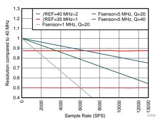
Figure 8. Effective Resolution Comparison for Various LDC Clocking Configurations
