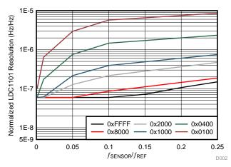
Figure 4. Normalized LDC1101 Resolution vs f<sub>SENSOR</sub> and RCOUNT
