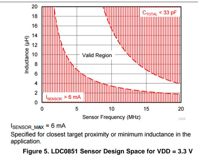
The LDC0851 may stay in an unresponsive constant HIGH or LOW (OUT, Pin 8) state when the sensor connected falls outside the design space.
