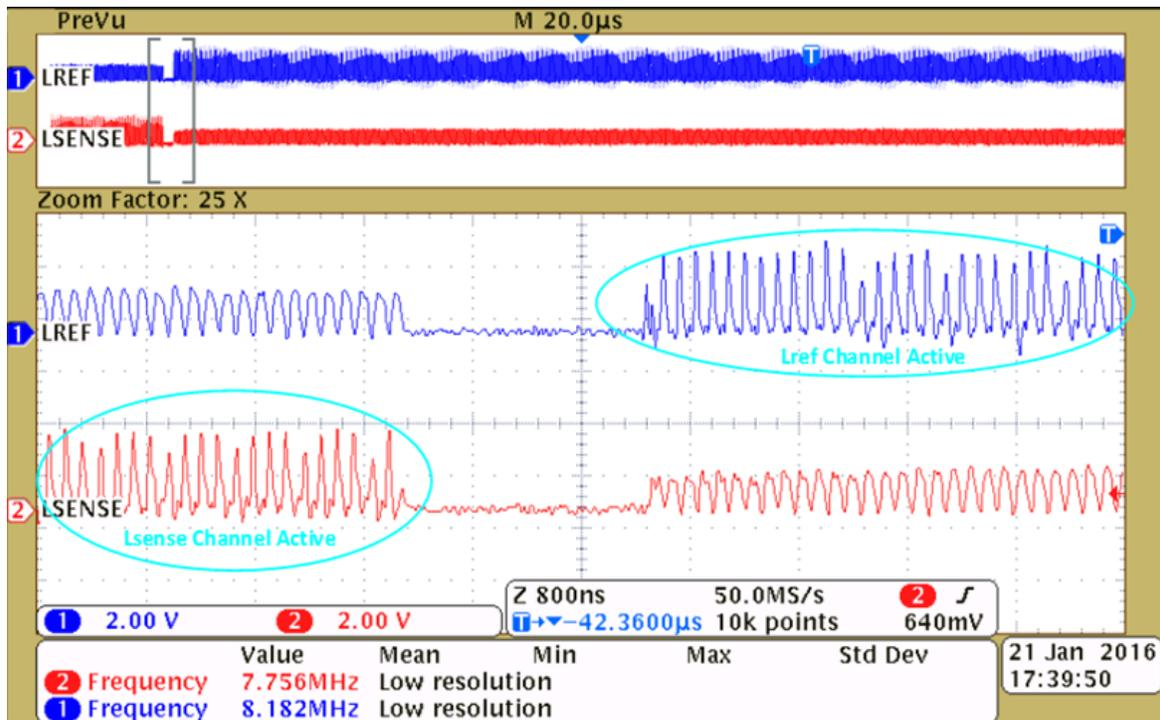
Figure 8. Figure 8: Sensor Capacitance Too High
