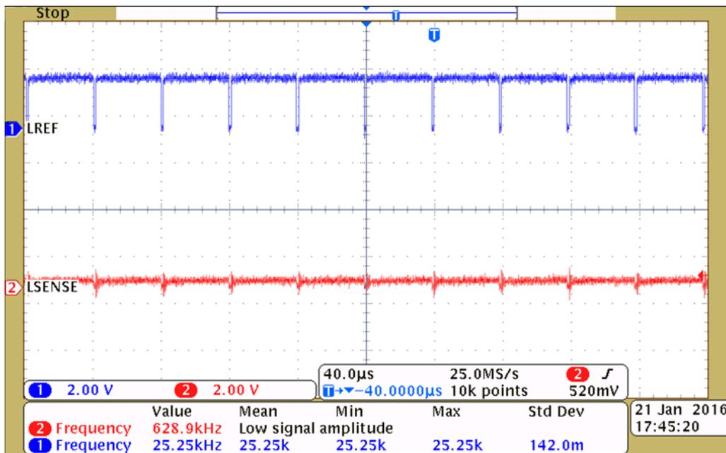
Figure 3. LREF Disconnected
