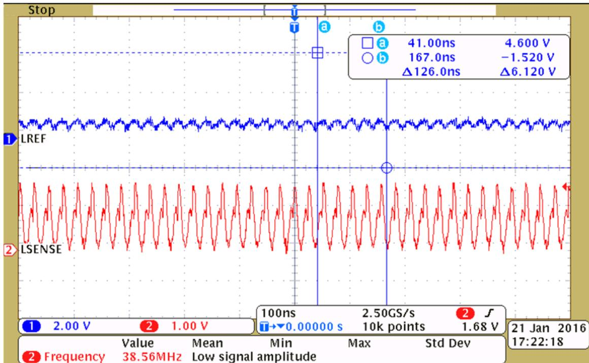
Figure 7. Incompatible Sensor, Sensor Inductance Too Low
