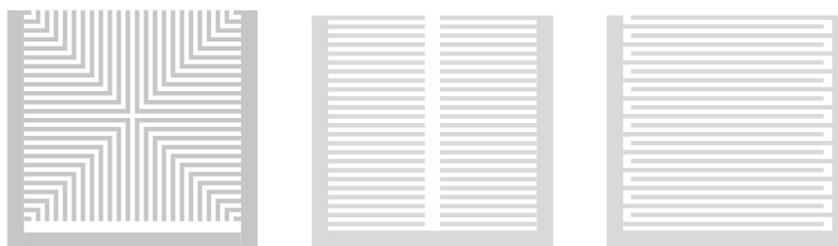
**Figure 2. Examples of Effective Coil Shielding Structures**
