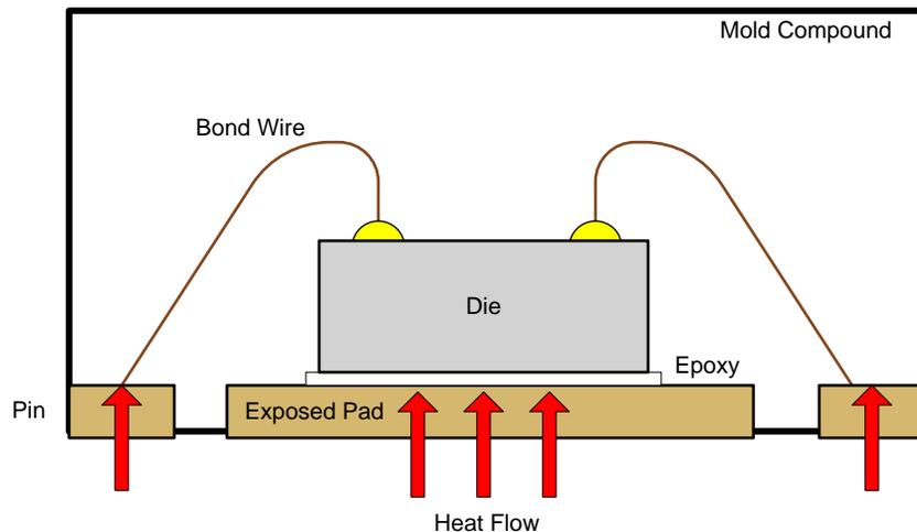
**Figure 1. Heat Transfer WSON (TMP116) Package Cross Section**
