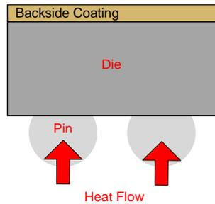
**Figure 2. Heat Transfer WCSP (LMT70) Package Cross Section**
