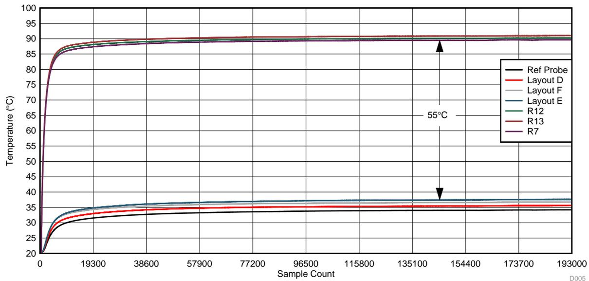
Figure 14. Layout D, E, F — 7.62-mm Distance
