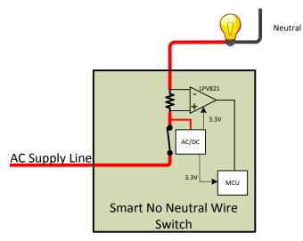
Figure 5. No-Neutral Switch Block Diagram With the LPV821
