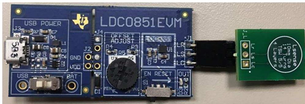
Figure 17. Prototyping Stacked Coils With LDC0851EVM
