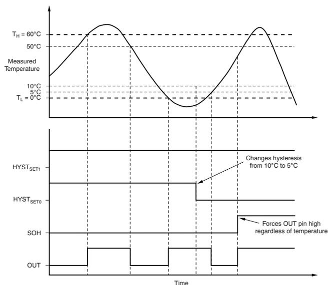
**Figure 2. Example Temperature Window Comparator Output Behavior**
