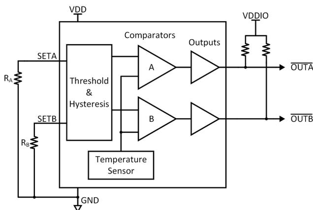
**Figure 3. TMP390 Block Diagram**
