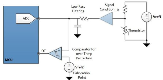
Figure 3. Example Discrete Implementation of a Temperature Monitor and Switch
