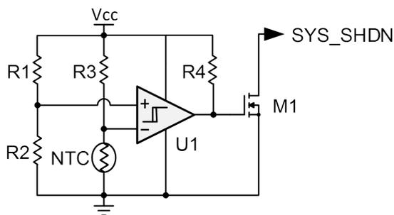
Figure 1. Example Discrete Implementation of a Temperature Switch
