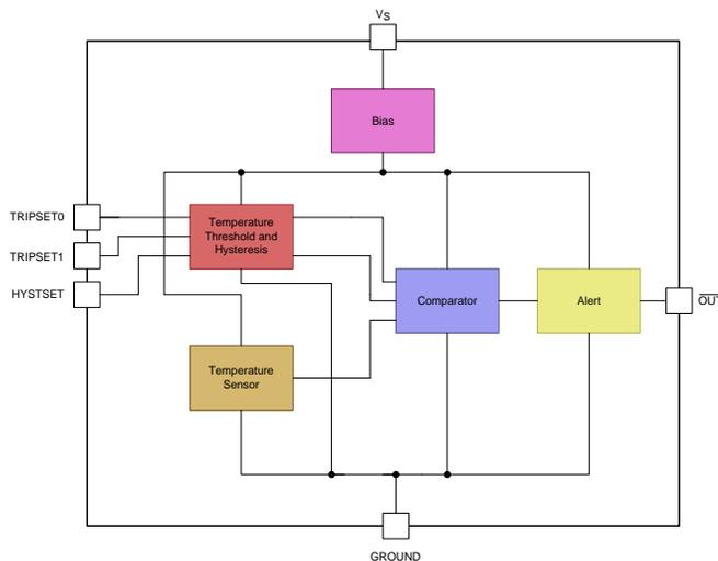
**Figure 4. Example Block Diagram of a Pin-Programmable IC Temperature Switch**
