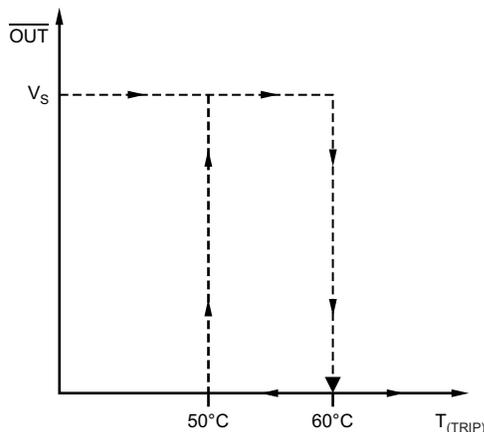
Figure 2. Example Temperature Switch Trip Behavior With Hysteresis
