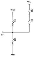
$$\frac{V_{PU} - V_H}{R_3 + R_4} + \frac{V_{REF} - V_H}{R_1} = \frac{V_H}{R_2} \Rightarrow R_1 = \frac{V_{REF} - V_H}{\frac{V_H}{R_2} - \frac{V_{PU} - V_H}{R_3 + R_4}}$$
