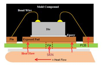
Figure 1. TMP116 Heat Flow Path
