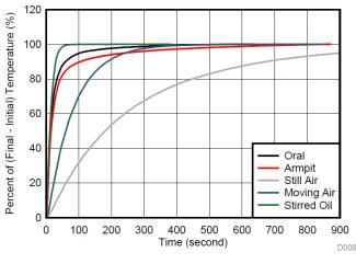
Figure 6. Thermal Response Comparison for Different Mediums
