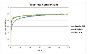
Figure 5. PCB Substrate Thermal Response Comparison
