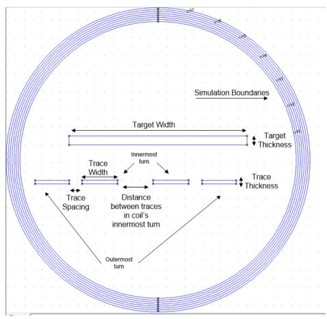
Figure 2-2. Example Planar Problem Workspace With Labeled Traces and Target
