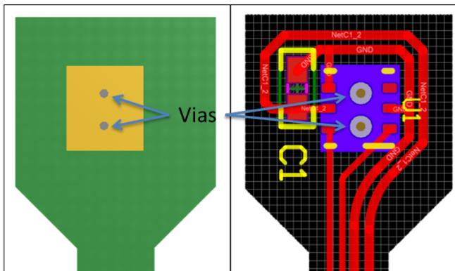
**Figure 3. Copper pour underneath TMP117 (Left), top side layout for TMP117 (U1, Right). The vias underneath the TMP117 and the copper pour provide a thermal path between the patient's skin and the device.**
