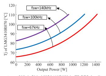
Figure 3-3. Junction Temperature of High-Side LMG3410R070 in TP PFC Applications at 400-LFM Cooling
