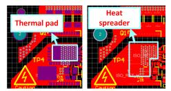
Figure 2-1. Thermal Pad of LMG341X GaN Power Stage and Top Copper Layer Heat Spreader of LMG3410R050-HB-EVM
