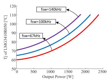
Figure 3-6. Junction Temperature of High-Side LMG3410R050 in TP PFC Applications at 400-LFM Cooling
