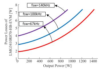
Figure 3-2. Power Losses of LMG3410R070-HB-EVM Board for TP PFC Applications at 400-LFM Cooling
