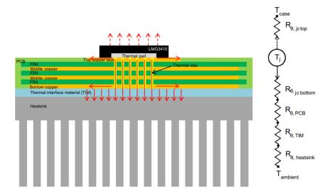
Figure 1-1. QFN Package on a PCB (Green), TIM (Blue) and Heat Sink (Gray)
