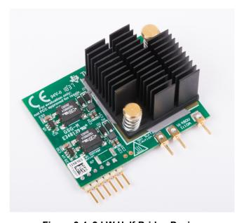
Figure 3-4. 2-kW Half-Bridge Design
