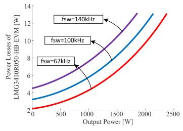
Figure 3-5. Power Losses of LMG3410R050-HB-EVM Board for TP PFC Applications at 400-LFM Cooling
