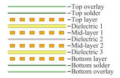
Figure 2-2. An Example Layer Stack of a 4-Layer Board
