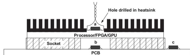
**Figure 4. Sensor Placement for High-Performance Processor Temperature Monitoring**
