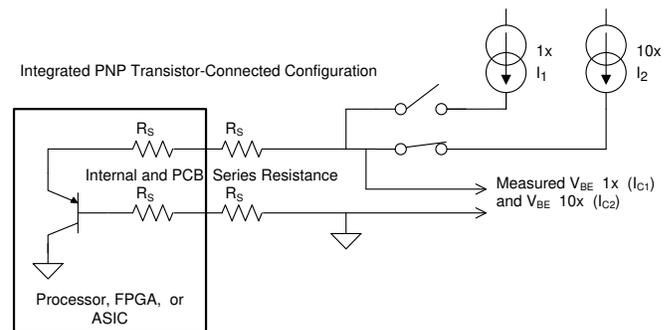
Figure 3.  $\Delta V_{BE}$  Measurement With Two Currents
