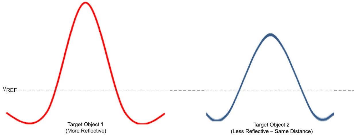
**Figure 3-4. Reflectivity and Its Effect on Input Overdrive**
