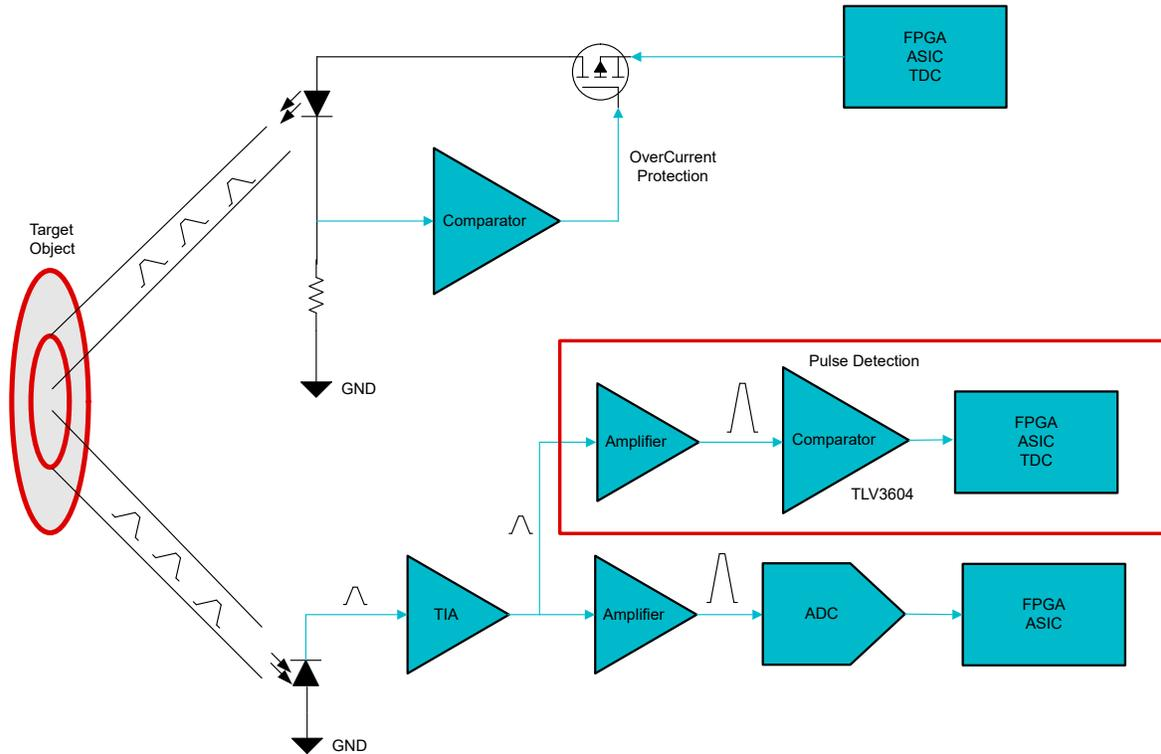
Figure 2-2. Time-of-Flight Concept Diagram
