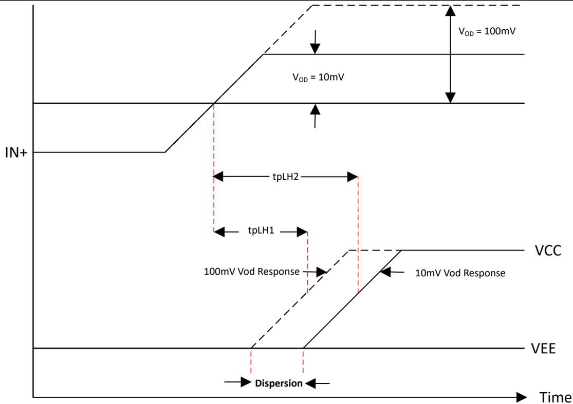
**Figure 3-2. Input Overdrive Dispersion Plot**
