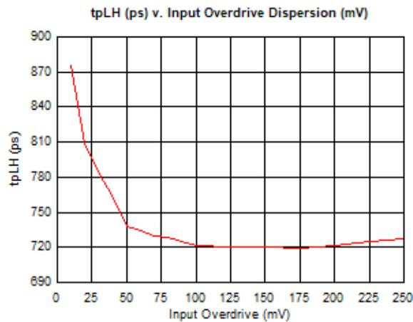
**Figure 3-3. Propagation Delay vs. Input Overdrive Dispersion**
