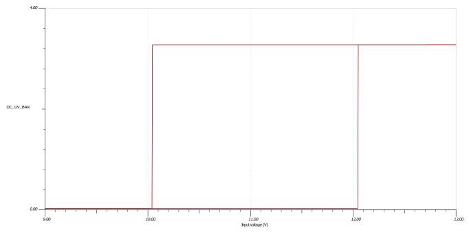
Undervoltage Test: Voltage Transfer Curve
