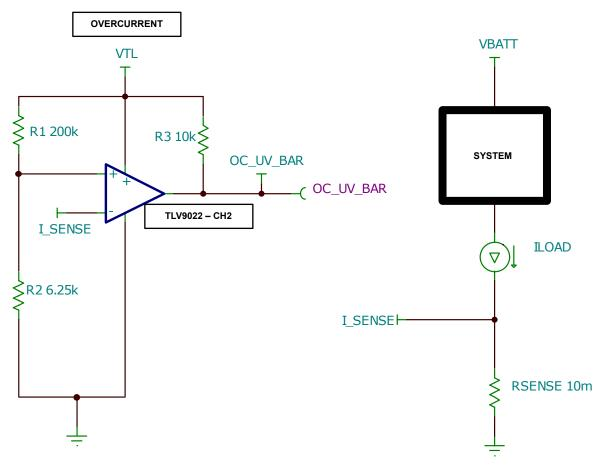
**Completed Overcurrent Protection Circuit With Simulated Load Current**
