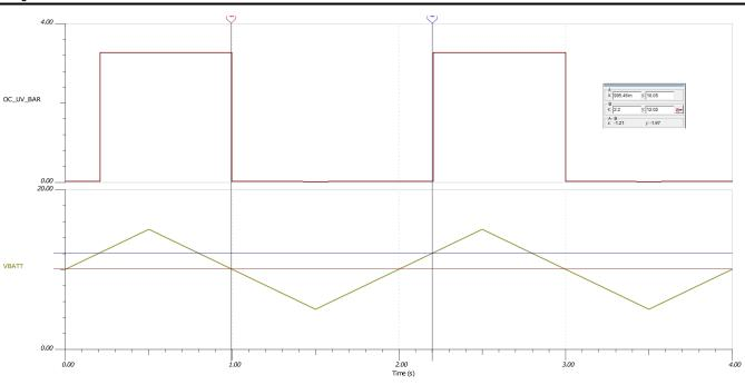
Undervoltage Test: Voltage Generator Across Load Spanning from 15-V to 5-V
