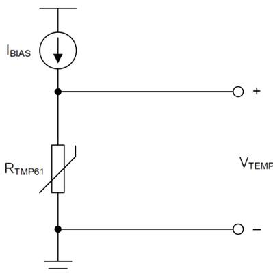
Figure 2-6. TMP61 Current Biasing Circuit
