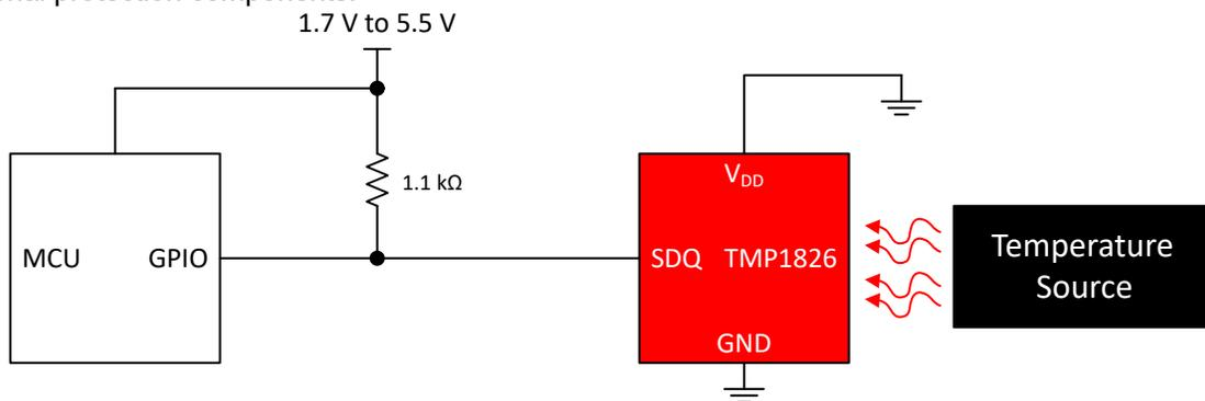
Figure 2-3. TMP1826 Bus Powered Application
