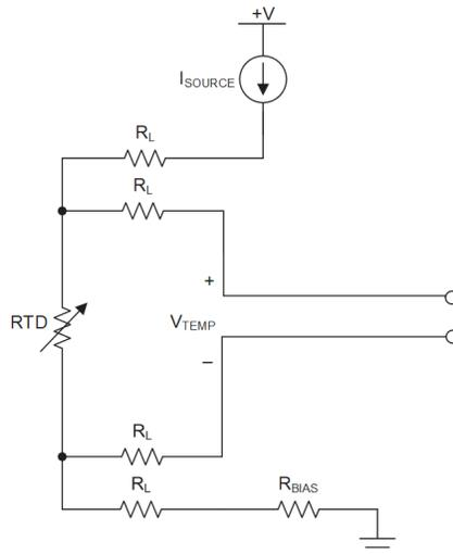
**Figure 1-3. Four-Wire RTD Configuration**
