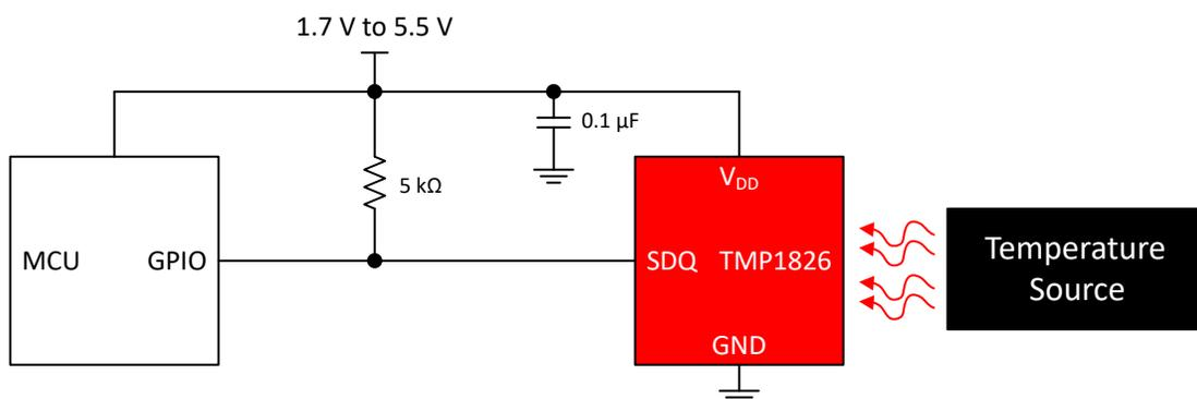
Figure 2-4. TMP1826 Supply Powered Application
