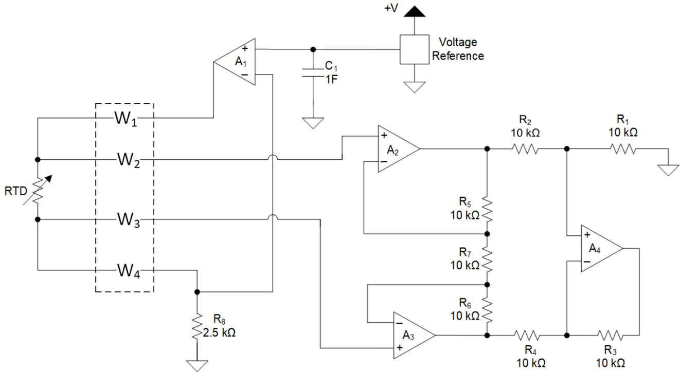
**Figure 1-5. Example of RTD Error Minimization Circuitry**
