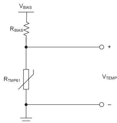
Figure 2-7. TMP61 Voltage Biasing Circuit
