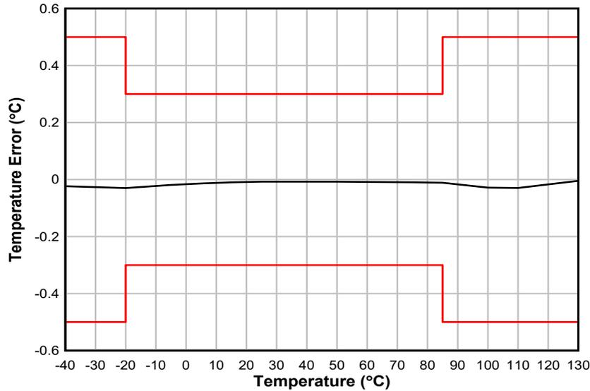
Figure 2-5. TMP1826 Temperature Error vs Temperature
