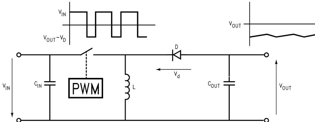
Figure 1. Basic Configuration of a Polarity Inverting Converter (Buck-Boost Converter)
