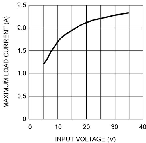
Figure 5. LM2673 Input Voltage vs. Load Current ( $V_{OUT} = -5\text{ V}$ ,  $L = 33\mu\text{H}$ )
