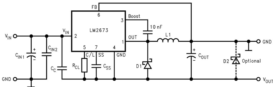
Figure 2. LM2673 Positive to Negative Converter
