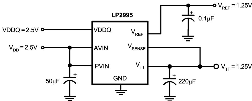
Figure 1. Implementation of Stub Series Termination Logic
