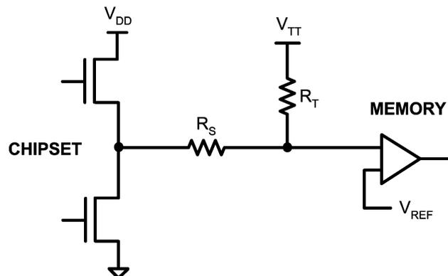
Figure 3. LP2995 Typical Application Circuit
