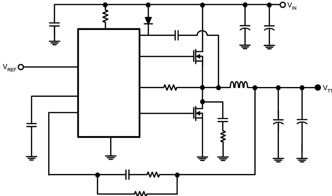
**Figure 2. Synchronous PWM Switcher Topology**
