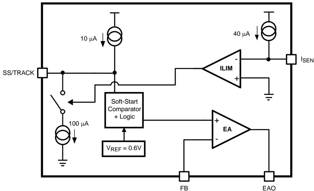
Figure 2. Error Amplifier and Current Limit Block Diagram
