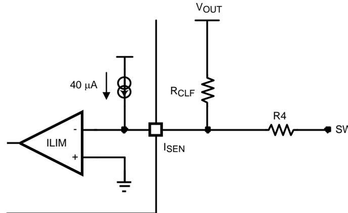
**Figure 4. Location of the Current Limit Foldback Resistor**
