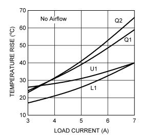
Figure 3. Temperature Rise at  $48V_{\text{IN}}$  with 6  $\mu\text{H}$  Cooper Inductor
