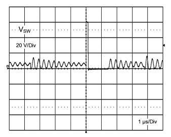
Figure 10. Discontinuous Operation using Diode Emulation Mode at 60V<sub>IN</sub> with JMP1 Installed
