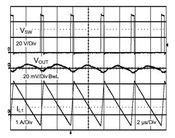
Figure 9. Full Synchronous Operation at 48V<sub>IN</sub> with JMP1 Removed
