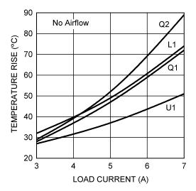
Figure 4. Temperature Rise at 48V<sub>IN</sub> with 5.6 µH Pulse Inductor
