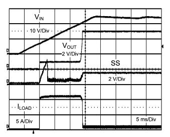
Figure 12. Start-up into Active Load at  $24V_{IN}$
