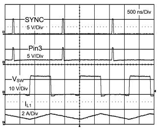
Figure 8. Synchronization at  $12V_{IN}$
