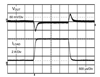
Figure 11. Transient Response at 24V<sub>IN</sub>
