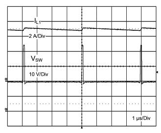
Figure 5. Short Circuit at 24V<sub>IN</sub> Room Temperature
