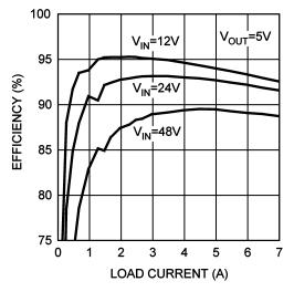
Figure 1. Efficiency with 6 µH Cooper Inductor
