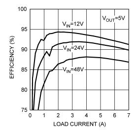
Figure 2. Efficiency with 5.6 µH Pulse Inductor
