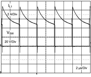
Figure 6. Short Circuit at 48V<sub>IN</sub> 125°C
