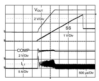
Figure 7. Short Circuit Recovery into Resistive Load with C7 = 1 µF and D2 Installed
