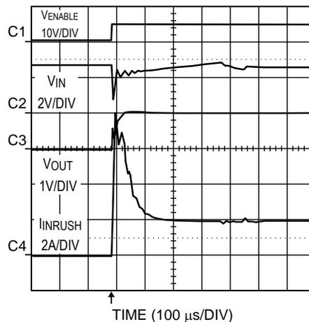
**Figure 3. Startup In-Rush Current Produces a  $V_{IN}$  and  $V_{OUT}$  Disturbance,  $C_{OUT} = 330\mu\text{F}$**
