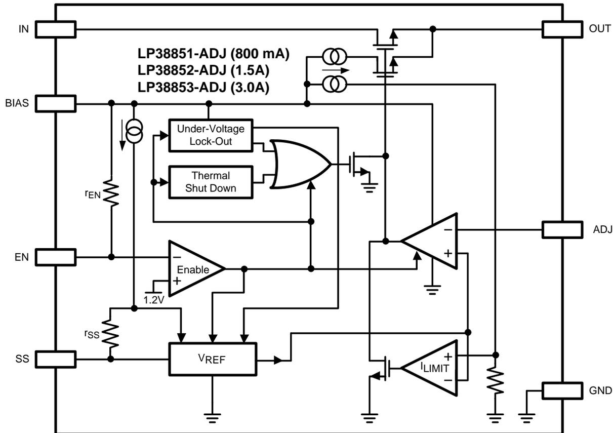
**Figure 1. LP38851/52/53-ADJ Block Diagram**
