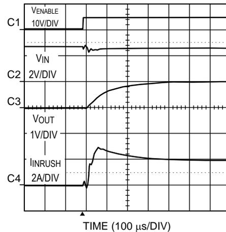
**Figure 4. Startup In-Rush Current With Soft-start,  $C_{OUT} = 330\ \mu\text{F}$**
