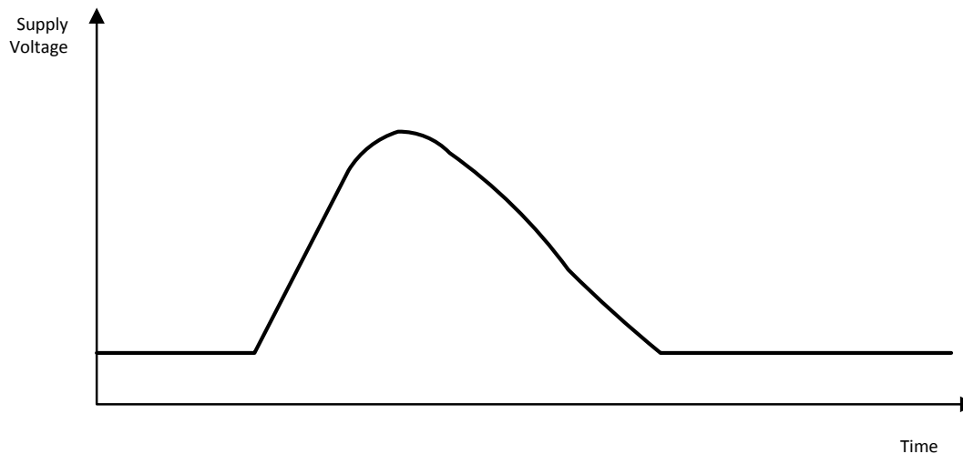
Figure 1. Typical Load-Dump Profile
