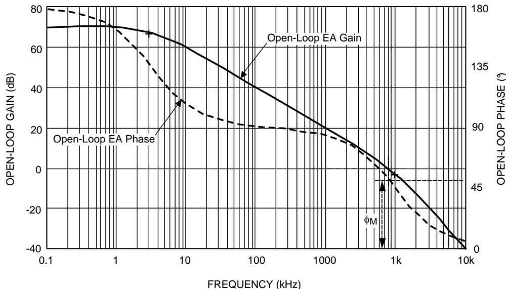
**Figure 2. Open-Loop EA Gain and Phase versus Frequency**
