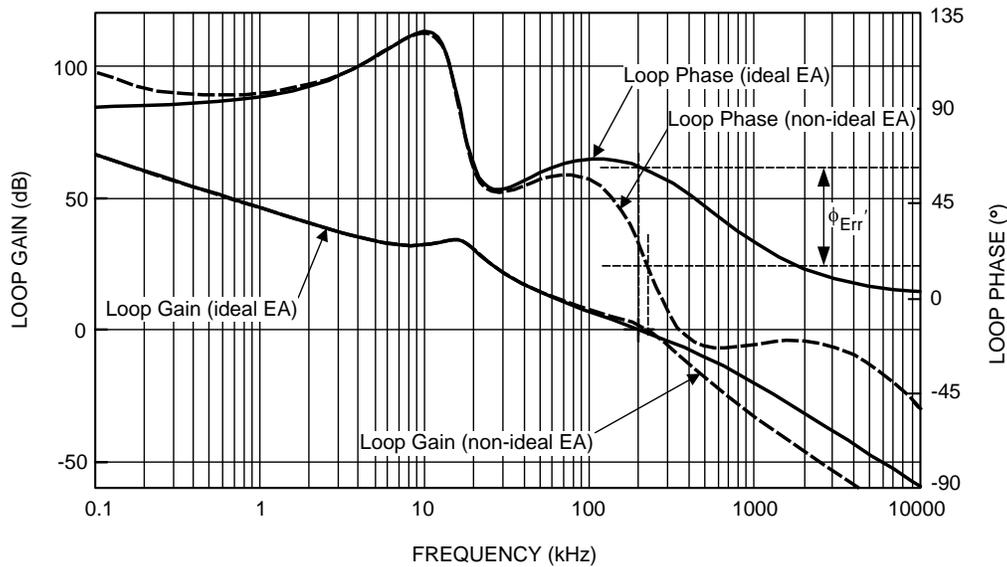
Figure 6. Overall Loop  $T_v(s)$  Bode Plot With Ideal and Actual EA
