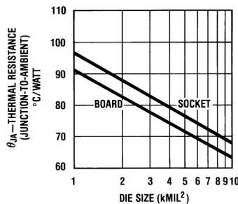
Figure 9. Thermal Resistance vs Board or Socket Mount
