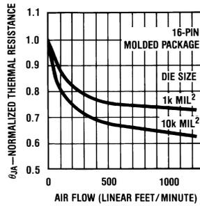
Figure 11. Thermal Resistance vs Air Flow (16-pin DIP)
