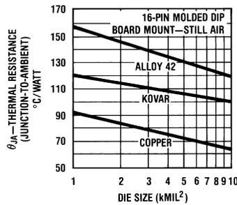
Figure 8. Thermal Resistance vs Lead Frame Material
