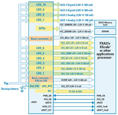
Figure 1. LP3970 Application diagram
