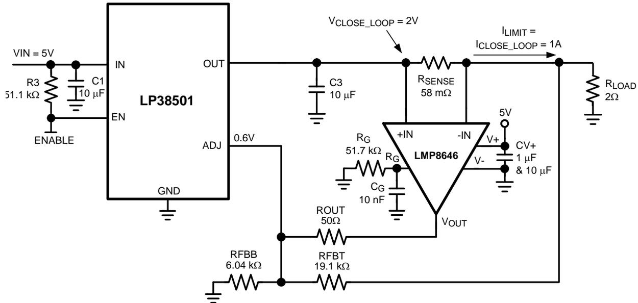
**Figure 1. Resistive Load Application with LP38501 Regulator**
