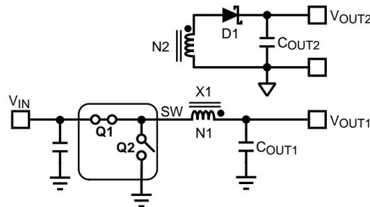
1b) An Isolated Buck Converter (Fly-buck)
