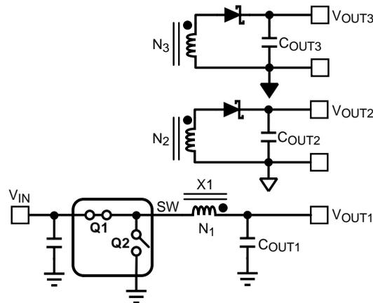
Isolated Buck Regulator with Three Outputs
