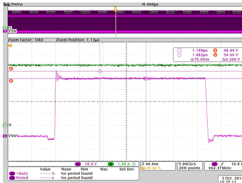
Figure 10. Switch Node Waveforms
