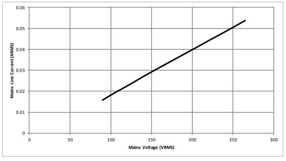
Figure 8. Line Current Vs Line Voltage
