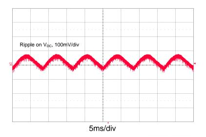
Figure 3. Voltage Ripple at V<sub>DC</sub>
