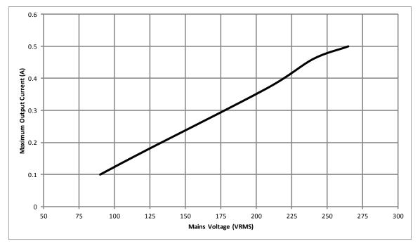
Figure 7. Max Output Current vs Line Voltage
