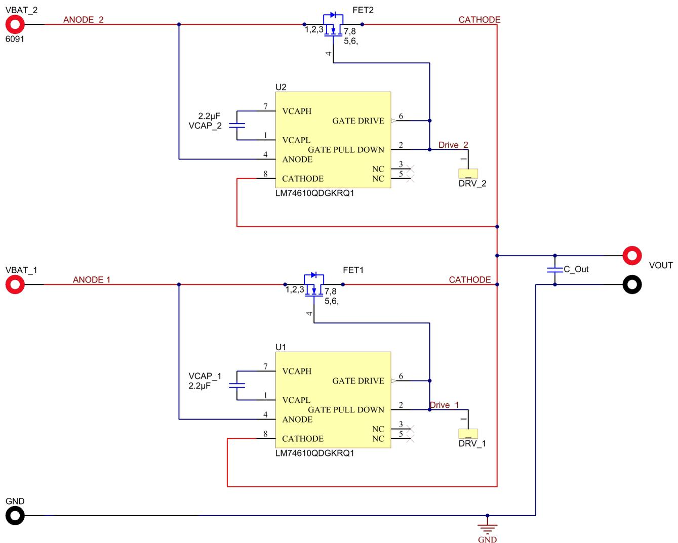
Figure 4. Schematic of LM74610-Q1 OR-ing Device
