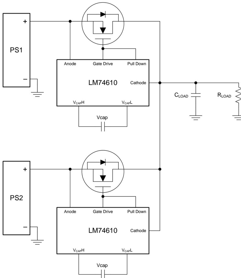
**Figure 2. Active OR-ing Application Circuit with LM74610-Q1**
