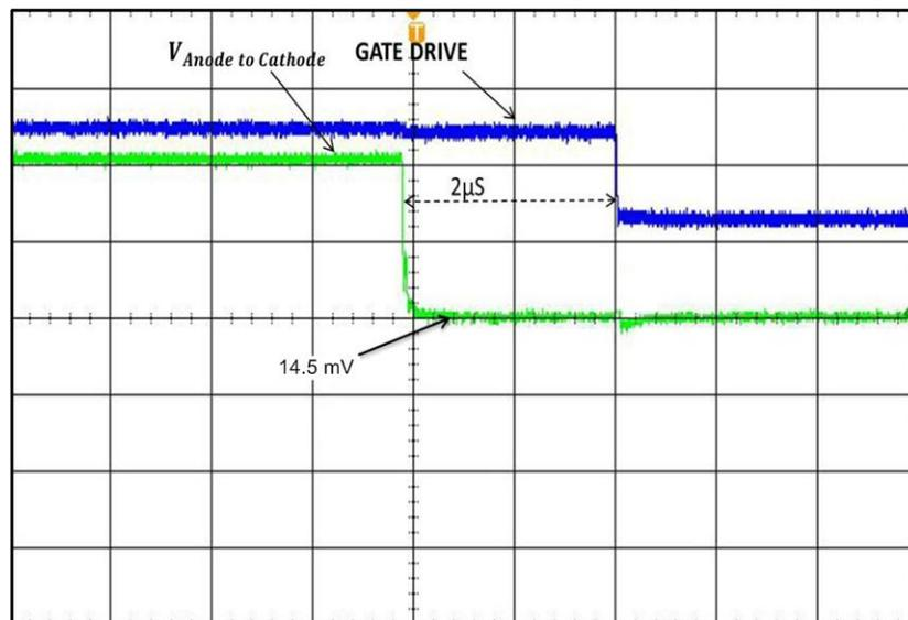
Figure 3. LM74610-Q1 Pull-Down Operation when Negative Polarity is Detected
