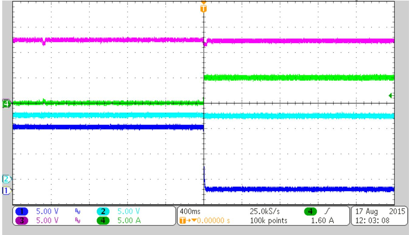
Figure 5. LM74610-Q1 OR-ing Device when PS1 Fails
