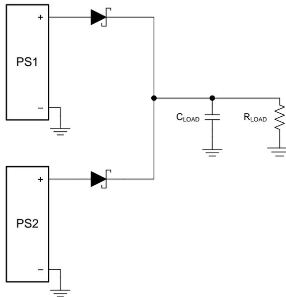
**Figure 1. Schottky Diodes Used for OR-ing**
