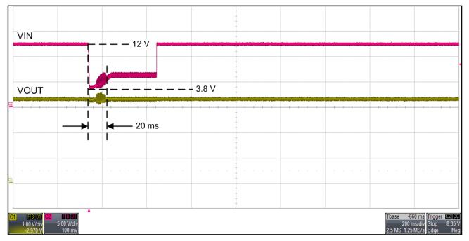
Figure 2. VOUT Regulated at 3.3V with VIN 3.8V for 20ms (Load 4A)
