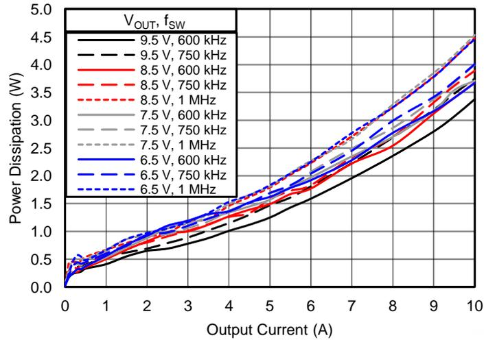
**Figure 2. Power Dissipation**
