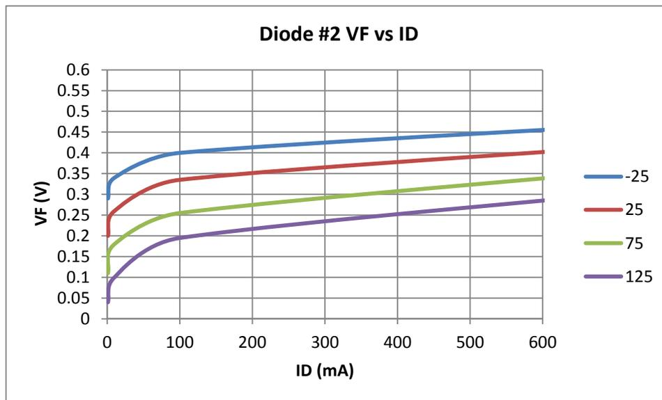
Figure 5. Diode #2 VF vs ID
