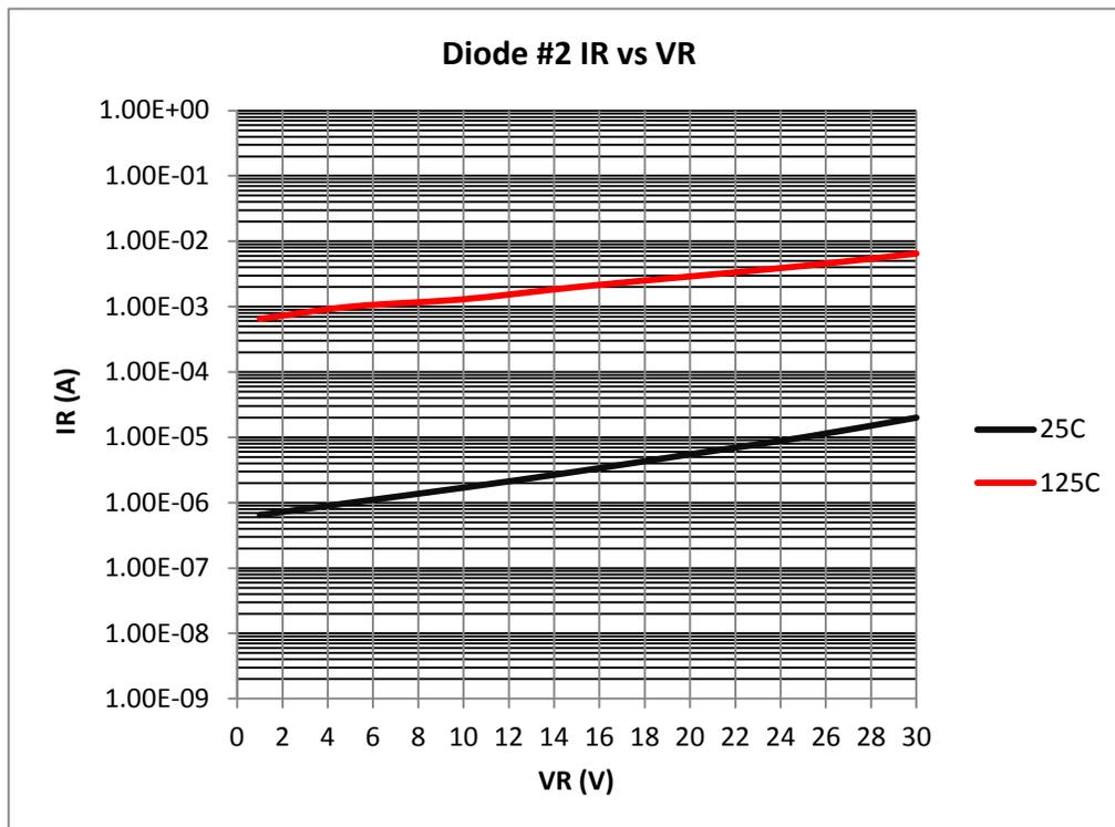
Figure 8. Reverse Leakage Current (Diode #2)
