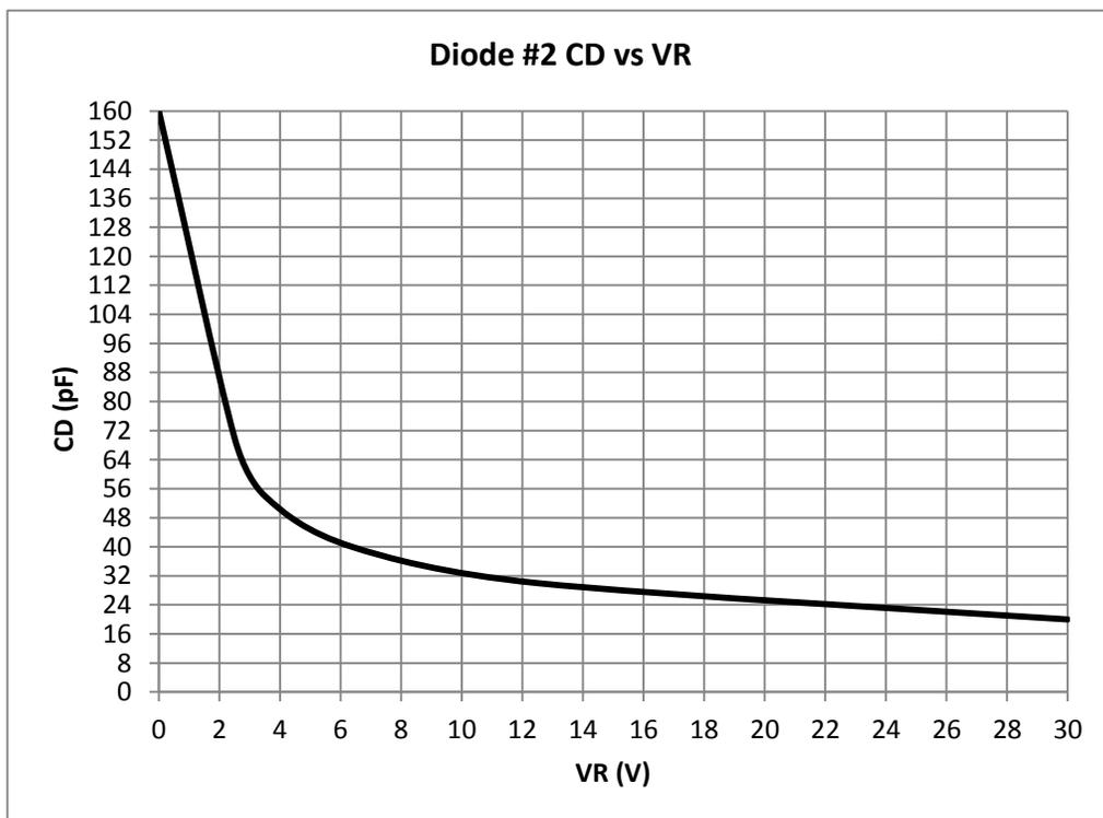
Figure 7. Diode Capacitance Curve (Diode #2)
