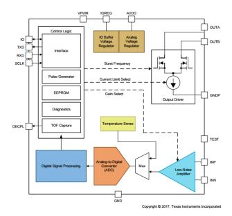
Figure 4. PGA460-Q1 Block Diagram
