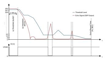
Figure 5. Time Command Interface and Threshold Comparator
