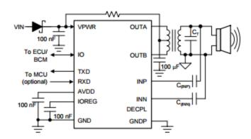
Figure 3. PGA460-Q1 Transformer Driven Schematic
