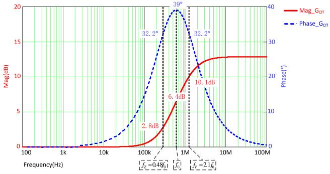
Figure 4. Bode Plot of Additional Transfer Function G<sub>cff</sub> When C<sub>FF</sub> = 10 pF
