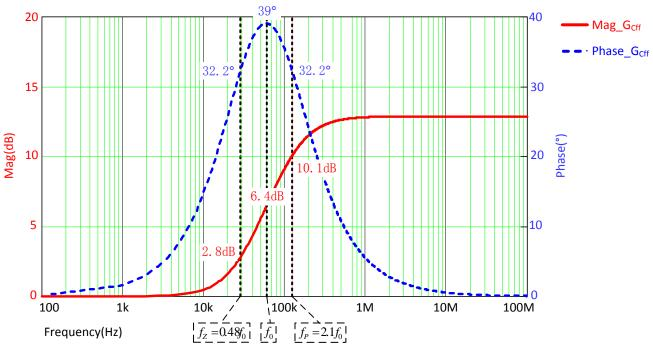
Figure 5. Bode Plot of Additional Transfer Function  $G_{Cff}$  When  $C_{FF}$  = 100 pF
