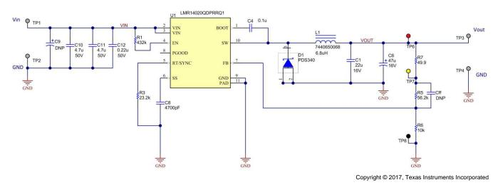
Figure 2. Original Schematic Without Feedforward Capacitor
