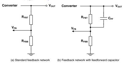
Figure 1. Feedback Network With and Without Feedforward Capacitor
