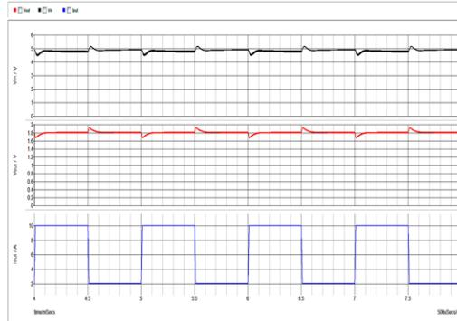
**Figure 22. Load Transient Test of Simplis Simulation**
