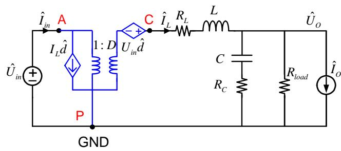
Figure 2. Buck Circuit Small Signal Model
