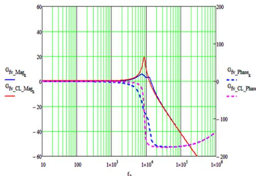
**Figure 15. Input Filter Frequency Response With Closed Loop**
