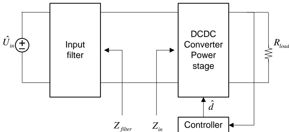
**Figure 8. Buck Control Block Diagram With LC Filter**
