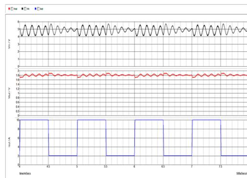
**Figure 17. Load Transient Test of Simplis Simulation**
