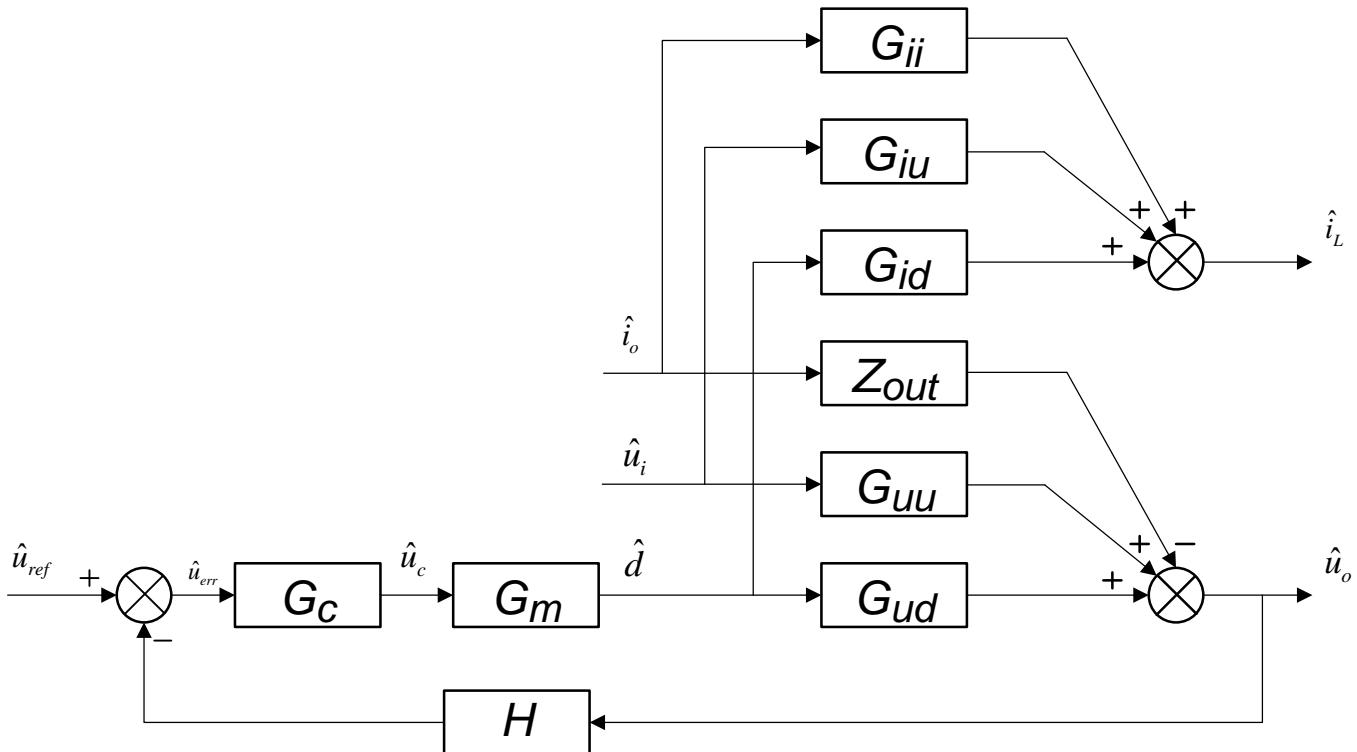
Figure 4. VMC Closed Loop Buck Controller Block Diagram
