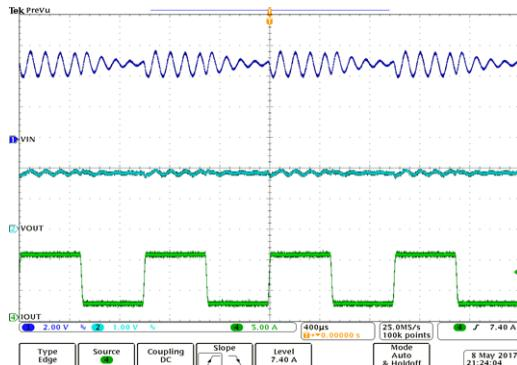
**Figure 16. Load Transient Test on EVM**
