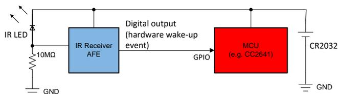
**Figure 1. Coin Cell Battery Powered IR Receiver**
