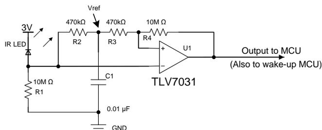
**Figure 2. IR Receiver AFE Using TLV7031 (Push-Pull Output)**
