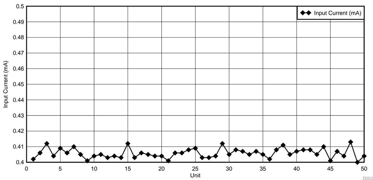
Figure 4. LM43603A-Q1 Input current at 8.5 V<sub>IN</sub> and 5 V<sub>OUT</sub> with 0.5-mA Standby load
