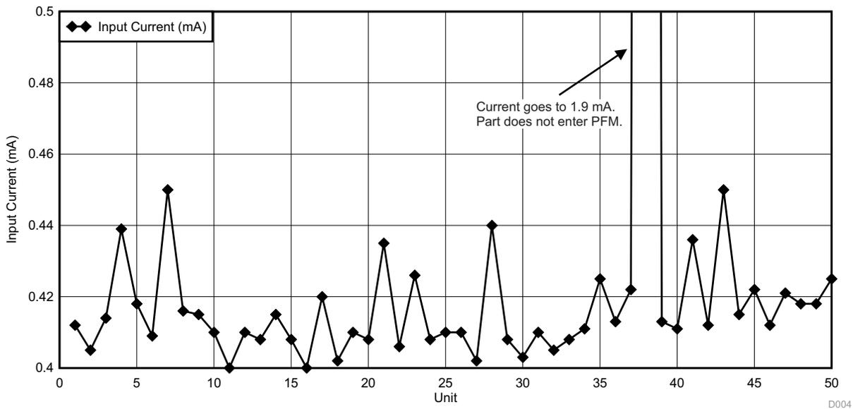
Figure 3. LM43603-Q1 Input Current at 8.5 V<sub>IN</sub> and 5 V<sub>OUT</sub> With 0.5-mA Standby Load
