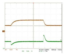
Figure 7. Load-Transient Performance
