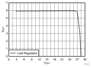
Figure 5. Load Regulation at 30  $V_{IN}$  With Increasing  $R_{LOAD}$  ( $V_{OUT}$  /  $I_{OUT}$ )
