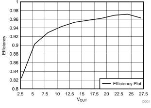
Figure 4. Efficiency at 30 V<sub>IN</sub>
