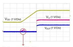
$V_{\rm G}$  rises up to ~400 mV because  $V_{\rm DD}$  is too low to pull  $V_{\rm G}$  to 0V
