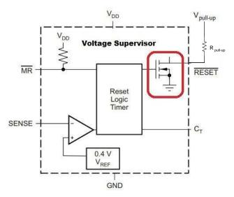
Figure 1. Voltage Supervisor Latch Circuit
