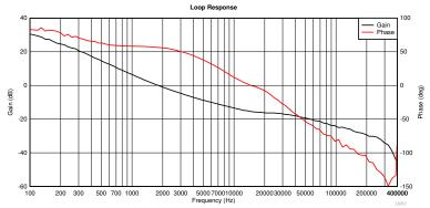
Figure 4-3. Control Loop Response  $V_{SUPPLY} = 4 V$ ,  $I_{LOAD} = 3 A$
