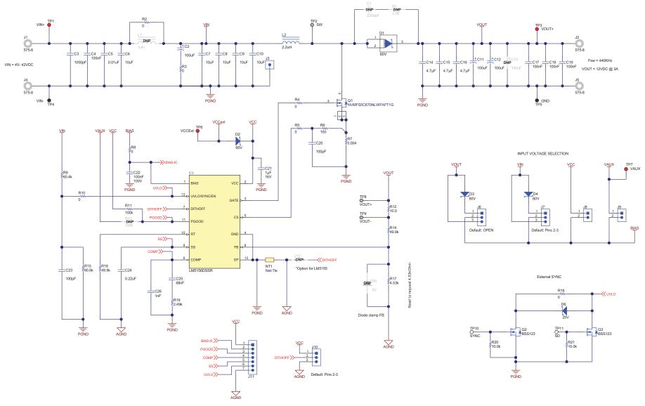
Figure 4-6. LM5156EVM-BST Schematic
