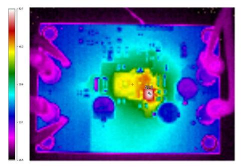
Figure 4-5. Thermal Image:  $V_{SUPPLY} = 4 V$ ,  $I_{LOAD} = 3 A$
