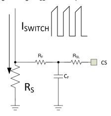
Figure 3-1. LM5156 Current Sense Network
