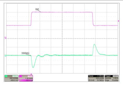
Figure 4-4. Load Step:  $I_{LOAD}1.5$  A to 3 A,  $V_{SUPPLY}$  = 4 V
