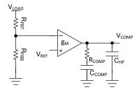
Figure 3-2. Type II Compensation Network
