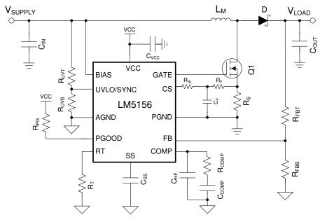
Figure 4-1. Application Circuit
