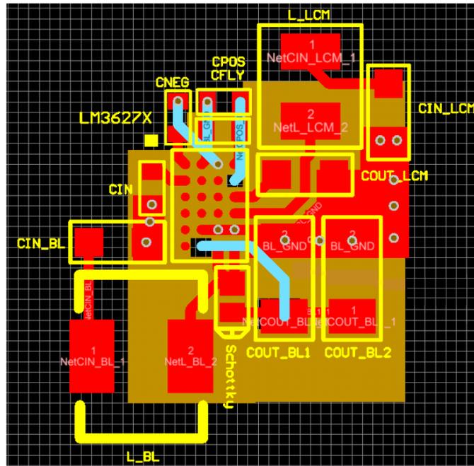
**Figure 8. LM36274 PCB Layout**
