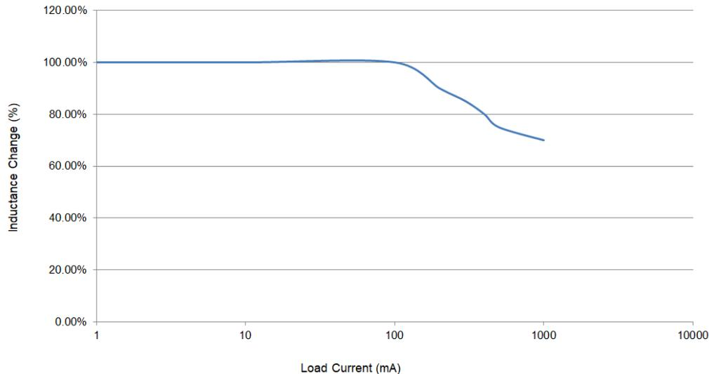
**Figure 7. Inductance vs Load Current**
