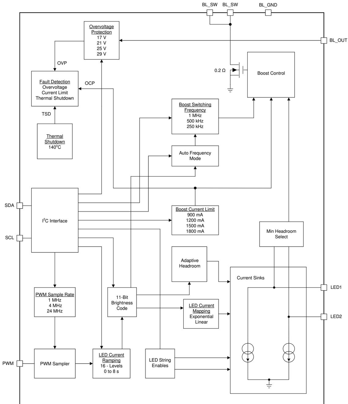
Figure 1. LM36273 LED Backlight Driver Unit
