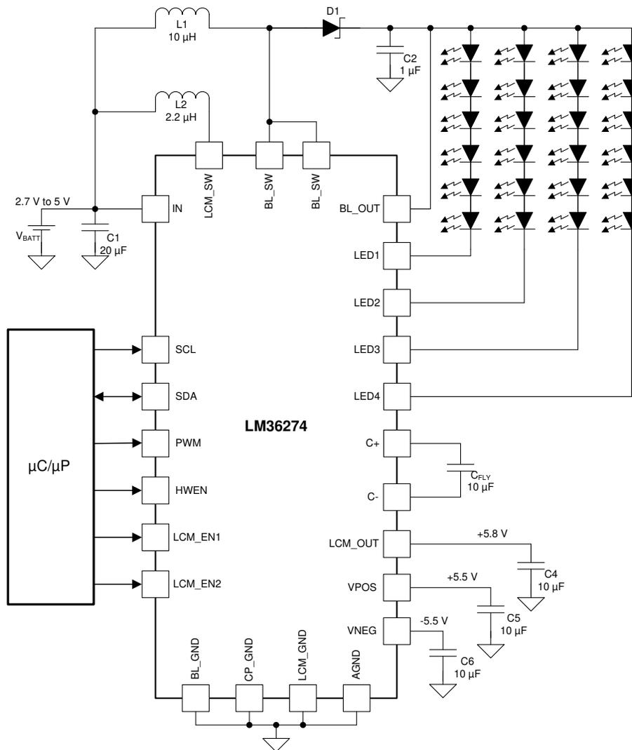
Figure 5. LM36274 Typical Schematic
