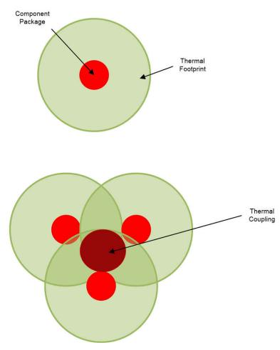
Figure 6-4. Example of Thermal Footprint Concept
