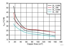
Figure 5-1.  $\theta_{JA}$  vs Copper Area for LM63635-Q1 WSON
