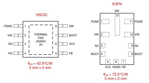
Figure 4-2. Comparison of HSOIC and VQFN Performance
