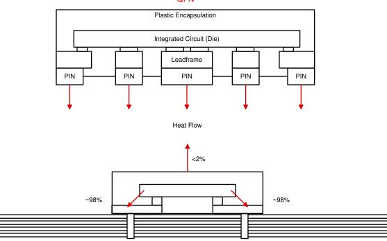
Figure 4-4. Typical Heat Flow in VQFN Package
