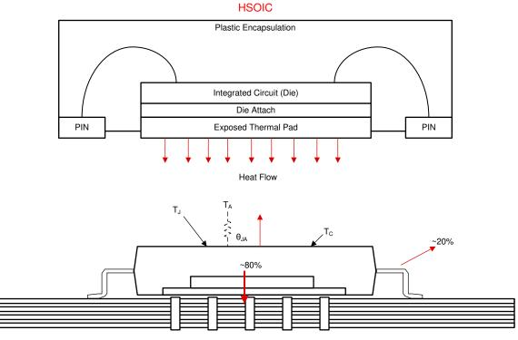
Figure 4-3. Typical Heat Flow in HSOIC Package
