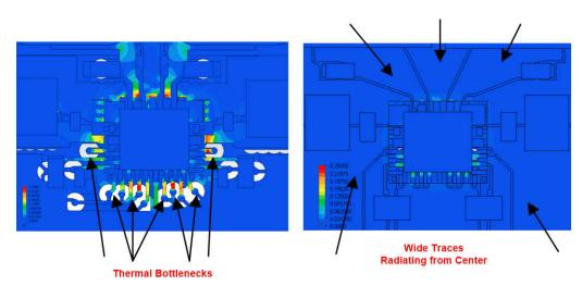
Figure 6-2. Comparison of Heat Flow Between Two PCB Layouts
