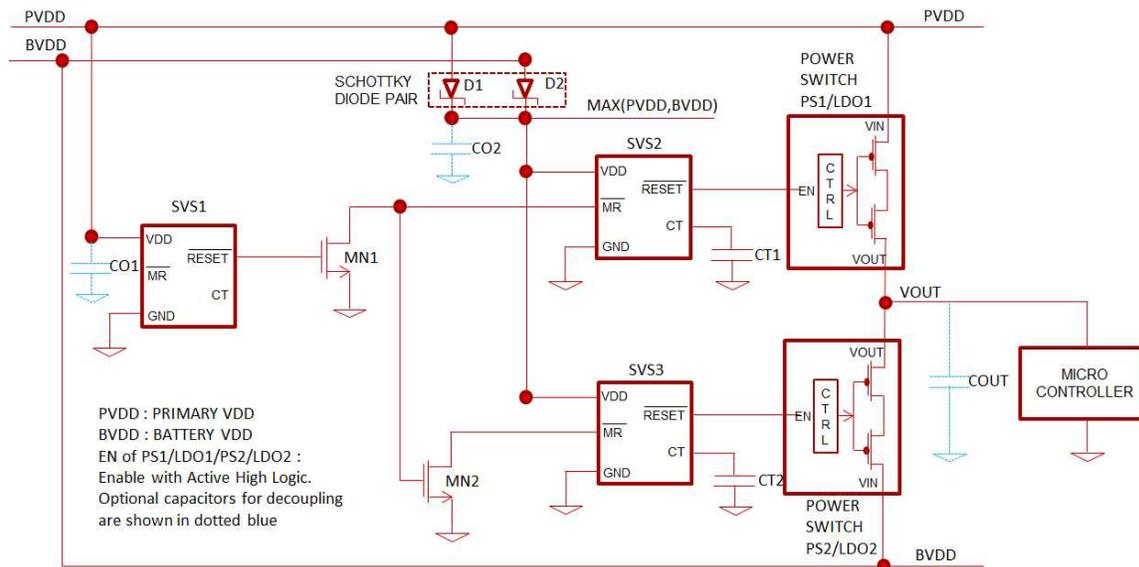
Figure 1. Back-up Battery Switchover Solution Block Diagram
