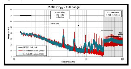
Figure 3-3. Conduction EMI Reduction by DRSS (LM5156, Switching at 2.2 MHz)
