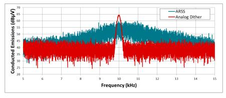
Figure 3-1. ARSS Improves Audible Noise by Spreading the 10-kHz Tone
